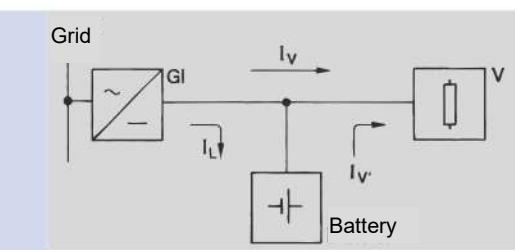
In case of **parallel operation** the consumer, DC-source and battery are working permanent in parallel. In case of standby-parallel mode (Online-mode) the DC-source must be able to supply permanently the battery and the consumer. The battery will be continuously fully charged and only releases the energy when the DC-source or the mains fails.
