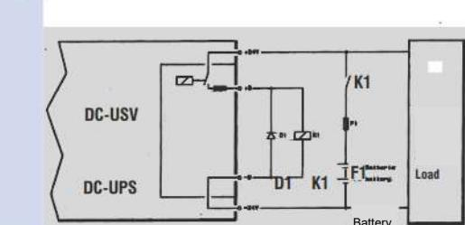
In **buffer-mode** the consumer power exceeds the rated power of the DC-source, so that the lacking power has to be summoned up by the battery. The battery is used to cover the peak load and is not continuously fully charged all the time. In case of a failure of the DC-source the battery will be switched to energize the consumers.
